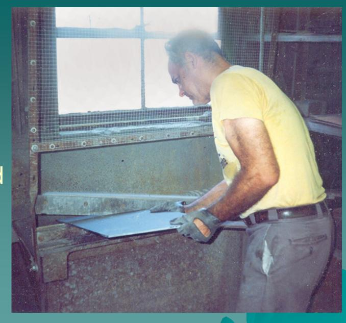
Nail holes are punched into the slates one at a time. Sometimes the slates are drilled.
